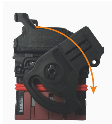
Figure: Rotating the latch
