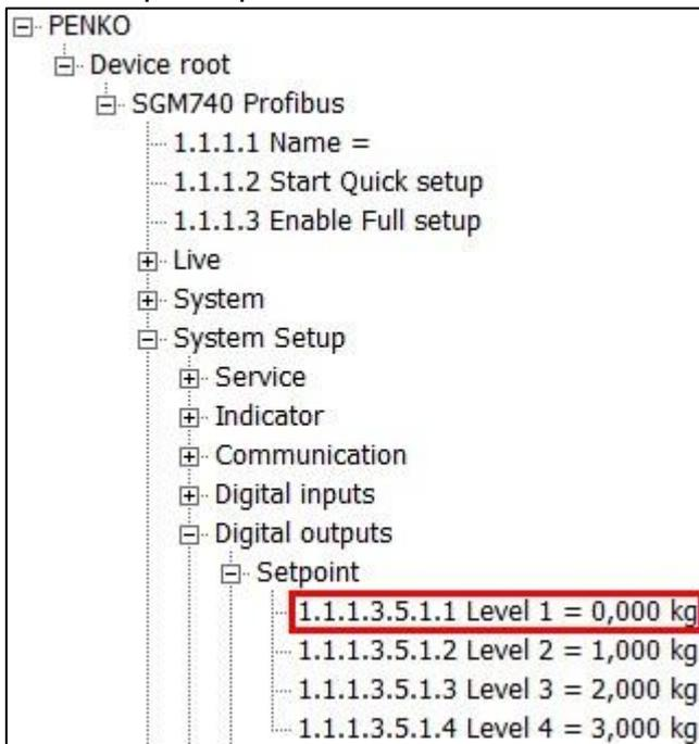
Setpoint 1 has path number 1.1.1.3.5.1.1. This results in the following input parameters:
