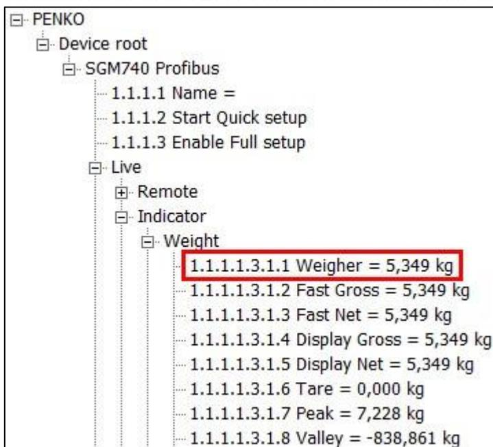
Weigher has path number 1.1.1.1.3.1.1. This results in the following input parameters:
