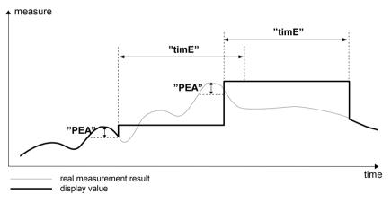
Figure 6.1. Process of peaks detection
