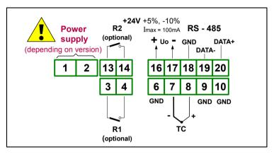
Figure 4.5. Terminals description (relay outputs)
