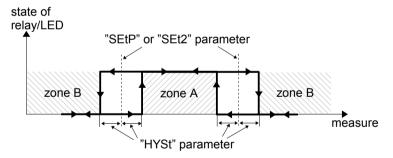
Figure 6.3. Two threshold control of the relay/LED outputs
