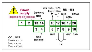
Figure 4.6. Terminals description (OC-type outputs)
