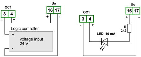
Figure 4.9. Example of OC-type outputs connection
