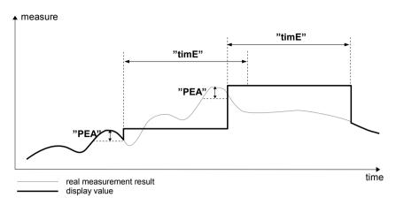
Figure 6.2. Process of peaks detection
