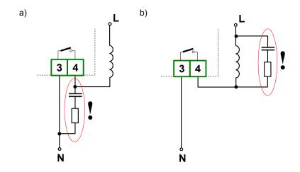
Figure 4.8. Examples of suppression circuit connection:
