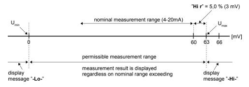
Figure 7.1 Example of definition of permissible range of input signal - "Hi r" parameter ("60" mode)
