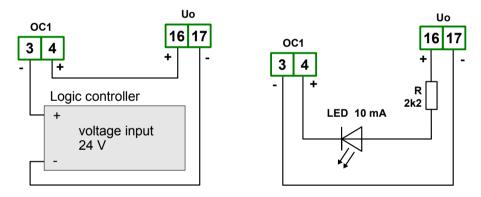
Figure 4.9. Example of OC-type outputs connection
