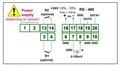
Figure 4.5. Terminals description (relay outputs)
