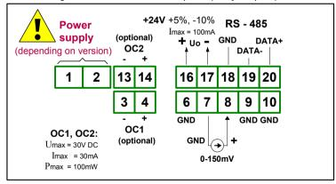
Figure 4.6. Terminals description (OC-type outputs)
