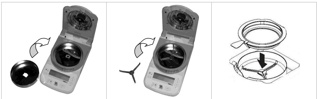
(1) Install and position Draft Shield
