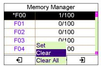
If the command "Clear All" is selected and confirmed, all data groups of the measuring instrument are deleted.
