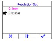
When the resolution is set to 0.01 mm, the surface of the test piece should be smooth to obtain accurate test results. When measuring rough surfaces or coarse-grained materials, it is recommended to use the low resolution.
