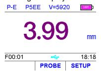
**Scan Mode** [Scan Mode]. In addition to the last thickness value measured, the minimum and maximum thickness values are also displayed during the measurement. By pressing, the minimum and maximum values are reset.
