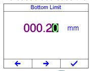
Press the key or the F3 key to confirm the setting. Press the key to cancel the change and exit the mode.
