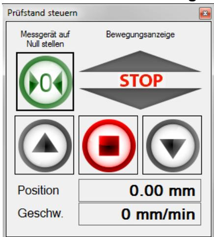
To enable a manual control of the measuring station using AFH LD, view the dialog box “Control of Measuring Station”. The dialog box can also be viewed by clicking View→Measuring Station in the main menu.
