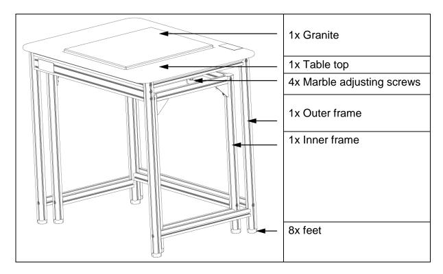
Figure 10 Final assembly drawing
