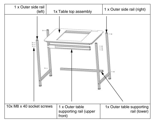
Figure 8 Outer frame assembly drawing
