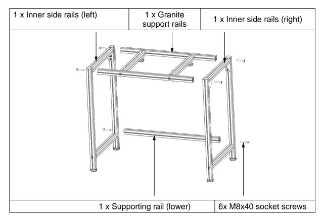
Figure 3 Inner frame assembly
