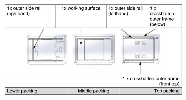
Figure 7 Outer frame packing
