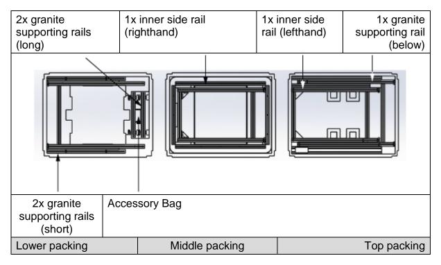
Figure 1 Inner frame packing
